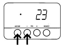
Remove the grille on speaker to access the controls. Push and hold AIR PAIR and VOL – button for 3 seconds to switch between Eco and Sleep mode.
