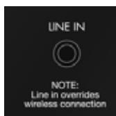
On rear panel of LV1 is a 3.5mm line input. Connect devices directly with cable. Connect iPod/iPhone/iPad dock, computer, cellphone, etc.
