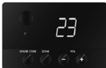
Under grille you will find display, IR receiver for remote, LED status indicator, volume, setting channel (House Code), and setting volume zone (Zone).
