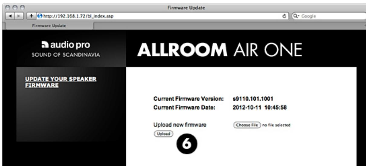
6. Select the firmware file (AirOne\_s9110.104.1001.fw) and press the UPLOAD button.
